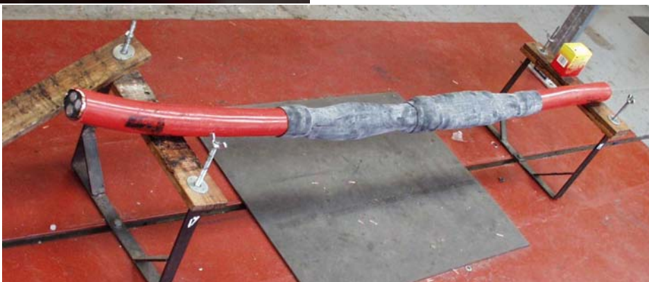
3 core polymeric to polymeric straight joint
